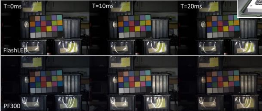
RGB Pixel Values: PF300 bulb versus FlashLED
