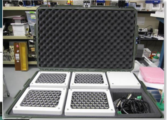
Battery-operated expeditionary package with 4 FlashLED units and battery power supply
